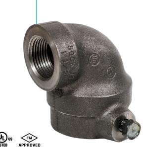
The Gruvlok Sock-It Piping Method provides a quick, secure and reliable method of joining plain-end steel pipe. Several Sock-It configurations are available: tees with NPT outlets, reducing run tees with NPT outlets, straight couplings, 90° elbows, straight tees and reducing elbows. Pressure energized elastomeric gaskets provide the Sock-It with a leak-tight seal. Specially designed lock bolts
